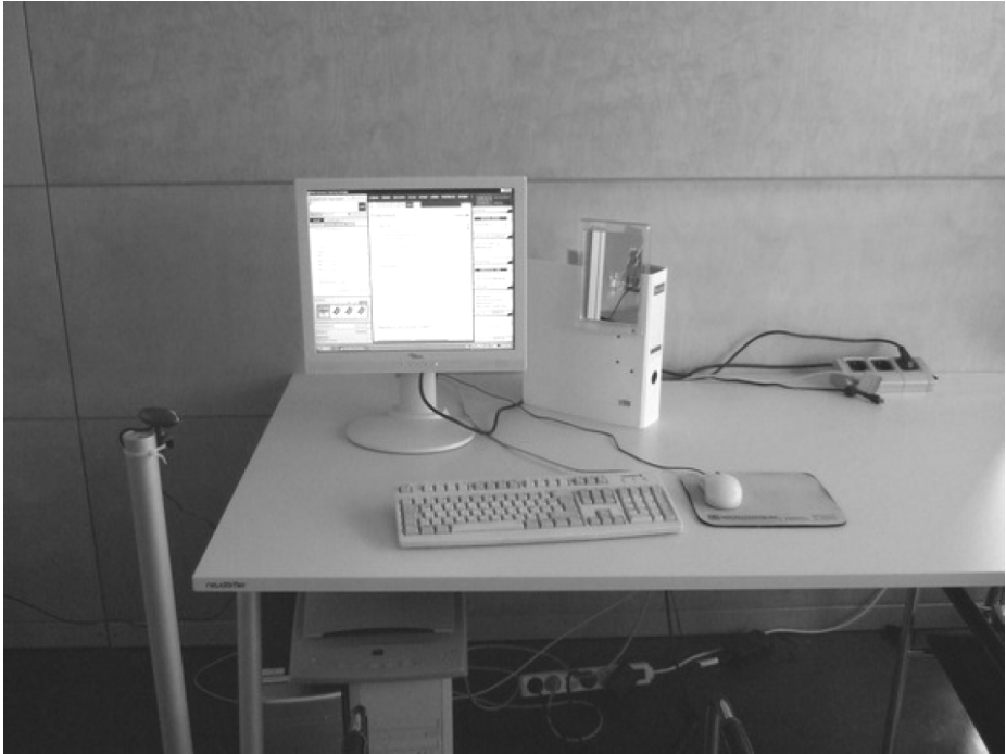
Fig. 3. Physical setup of the experiment: Camera and microphone ( left ), TFT display ( center ), mirror for capturing facial expressions ( right of display ), input devices ( in front of display )
